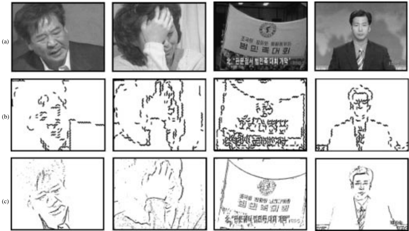
Fig. 16. Examples of extracted edge image from MPEG video data. (a) Original images, (b) example of extracted edge image using the proposed method, and (c) images which are filtered by the Sobel filter.
